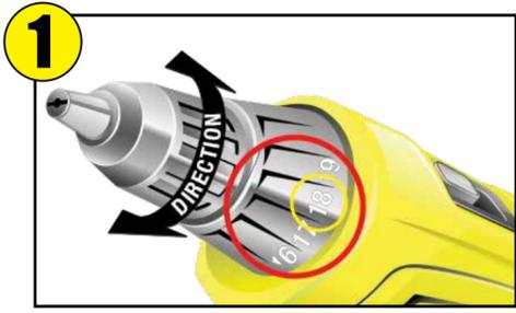
**1** **ALWAYS** check direction & clutch setting of the cordless drill before inserting into lower gearbox!
